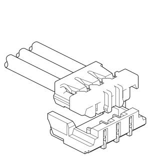
This ADH connector is compact and low profile type, height 1.9 mm and width 4.3 mm, 1.3 mm pitch wire-to-board connector.
