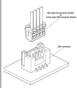
The SMT top entry type headers that can be mated with the 1.5 mm pitch CZ connector socket are on the lineup.
