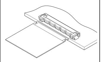
This is 0.5mm pitch connector for FPC which has the exclusive GND contact and enables high-speed transmission with connecting to the impedance controlled FPC. Adopting the auto lock mechanism that makes lock by performing the one action of snap-in-work, the workability improvement is realized.
