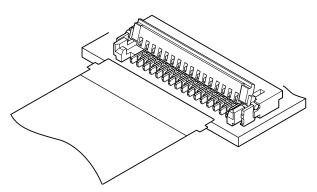
In addition to achieving space saving and low profile features, this connector is designed to be compatible with a FPC with protrusions, so that the FPC insertion process is simplified and malfunctions such as incomplete insertion or mis-insertion are prevented.
