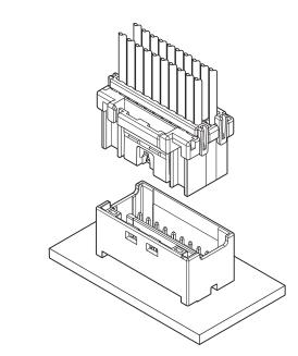
This PID connector is a 2.0 mm pitch box type wire-to-board connector with secure lock device, and it has the mechanism for detecting half mating, which is possible to judge electrically whether its state is the complete or incomplete mating by the circuit of detecting half mating provided at the part of connector.
