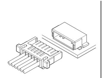
This is a wire to board connector with secure locking device used for power supply of LED.
