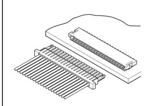
This is an ultra-thin 1.0 mm pitch wire-to-board connector for thinner and smaller devices, with a mounting height of 1.8 mm for the normal type and 1.4 mm for the offset type.
