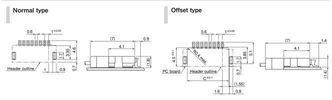
Note: 1. The figure of PC board layout is the figure viewed from the connector mounting side.
